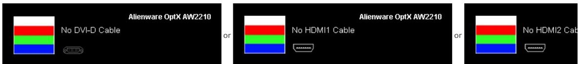
4. This box also appears during normal system operation, if the video cable becomes disconnected or damaged.
