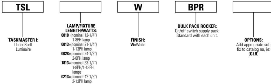
For electronic ballast, substitute **TSLP** for **TSL**, ie: **TSLP0018W BPR**.
