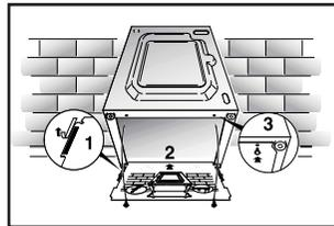
Level the machine using the 4 feet.
