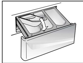
This special container must be inserted into the compartment marked "II" in the detergent drawer, also when you wish to use the "RINSE" programme as BLEACHING cycle.
