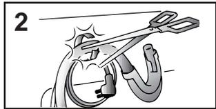
Carefully cut through the hose retaining clip at the rear of the appliance (diagram 2).
