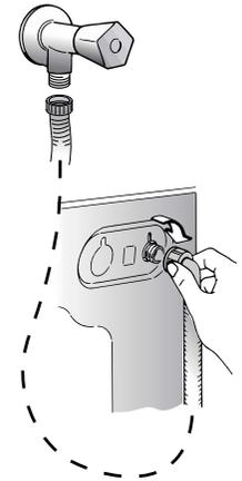
This machine only uses cold water, therefore only one hose is needed to connect to the cold water supply. Do not connect to the hot supply. Cold fill is an energy efficient system. Only the water required for the washing is heated. There is no loss of heat in the pipeline from a hot water tank or boiler to the machine.
