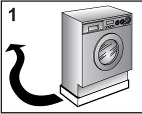
1 Remove the polystyrene base and place the machine near its permanent position (diagram 1).
