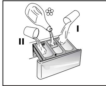
If liquid detergents are used, please insert the special container supplied into the compartment marked "II" in the detergent drawer. This ensures that the liquid detergent enters the drum at the right stage of the wash cycle.
