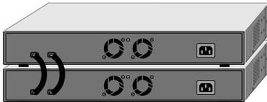
Figure 4-4. Cabling FS524S Stacked Switches
