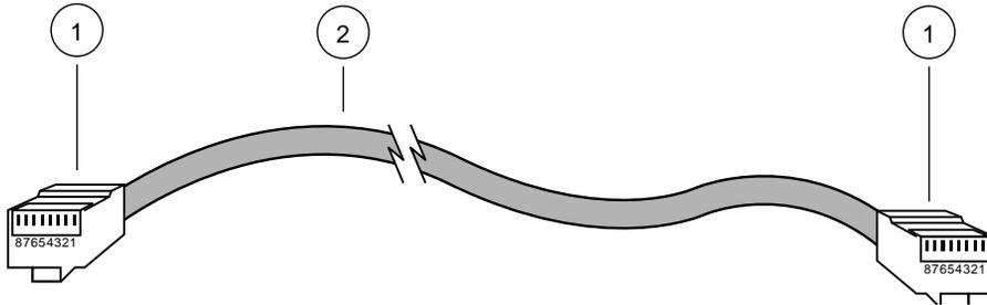
Figure C-3. Category 5 UTP Cable with Male RJ-45 Plug at Each End
