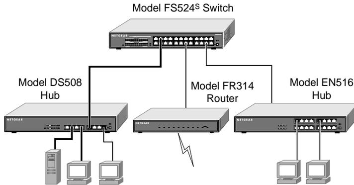
Figure 3-2. Example of Segment Switching and Bridging
