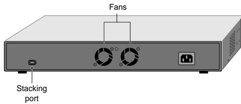
Figure 2-1. Front and Back Panels of the FS517TS Switch
