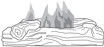
Figure 46 - Incorrect Burner Flame Pattern
