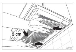
■ Tilt the front of the external filter slightly down and out.
