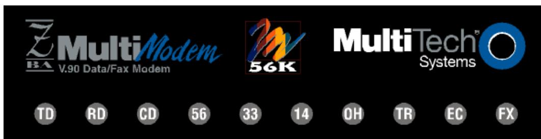
The MultiModemZBA LED indicators on the front panel indicate status, configuration, and activity:
