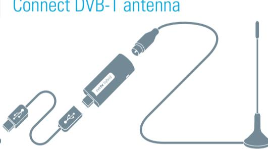
**EN****Connecting a rod antenna**
