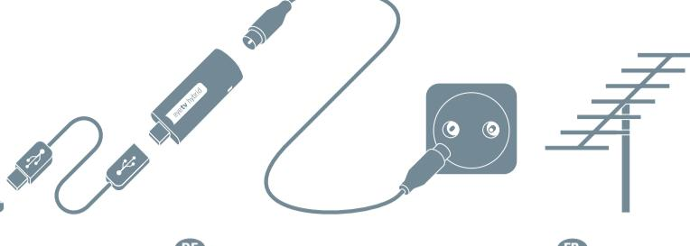
**EN****Connecting a roof antenna**
