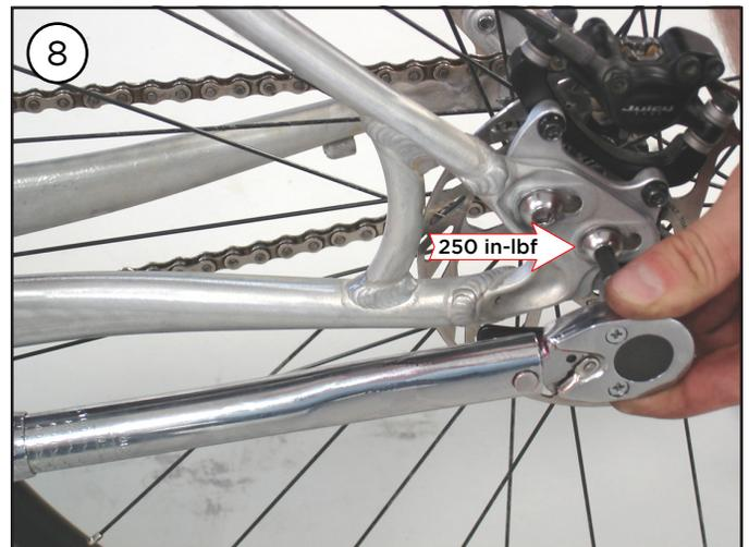
Torque the drive side and non-drive side bolts to 250 in-lbf.
