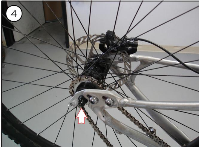
Install the rear wheel in the loose dropouts. Tightening the quick-release will self-align the wheel and dropouts.
