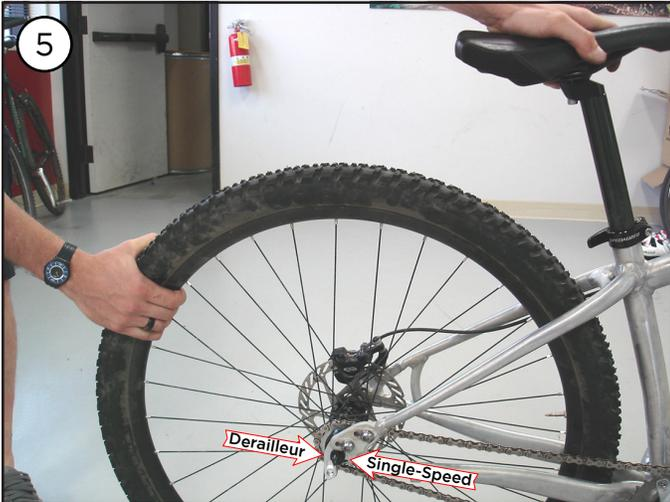
Single-Speed style: Pull the wheel backward, so that the chain is properly tensioned.
