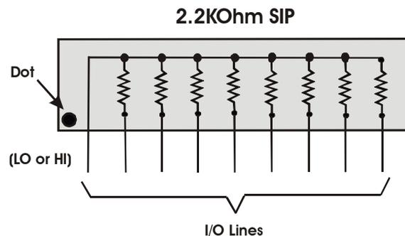
Figure 4-1. Eight-resistor SIP schematic
