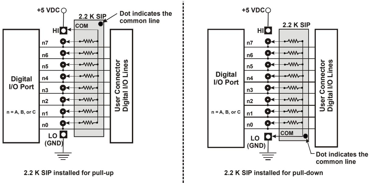
Figure 4-2. Pull-up and pull-down resistor SIP schematic
