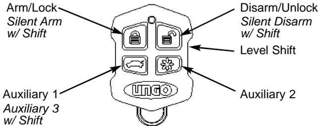
The Ungo MS2106 comes with 2 Random Code Remote Transmitters used to control the system's features. Each time a transmitter button is pressed, the LED will flash to indicate that a transmission is taking place.
