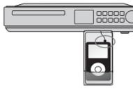
4. Press the FUNCTION button on the remote control or the CD-RADIO-AUX button to change to AUX. The AUX indicator lights up.
