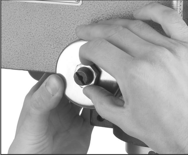
**Figure 43.** Loosening cover and jam nut
