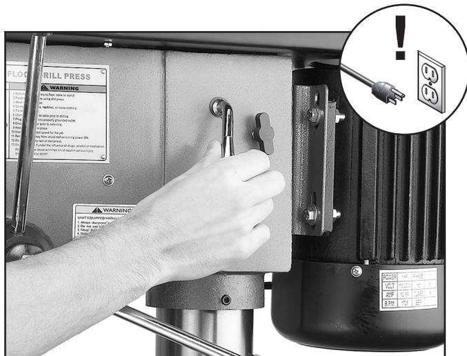
**Figure 27.** Using the belt tension lever.
