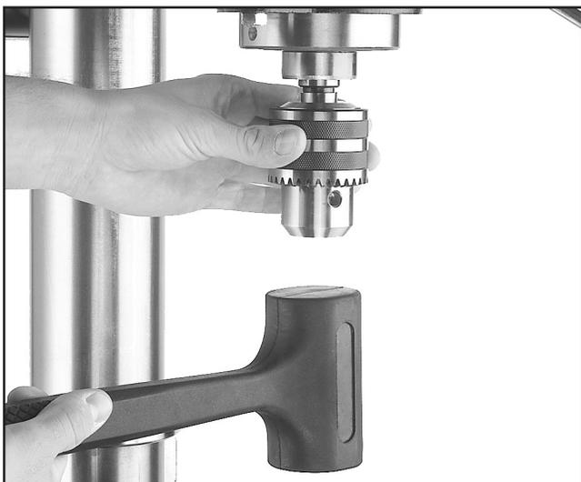
**Figure 17.** Seating arbor and chuck into spindle.
