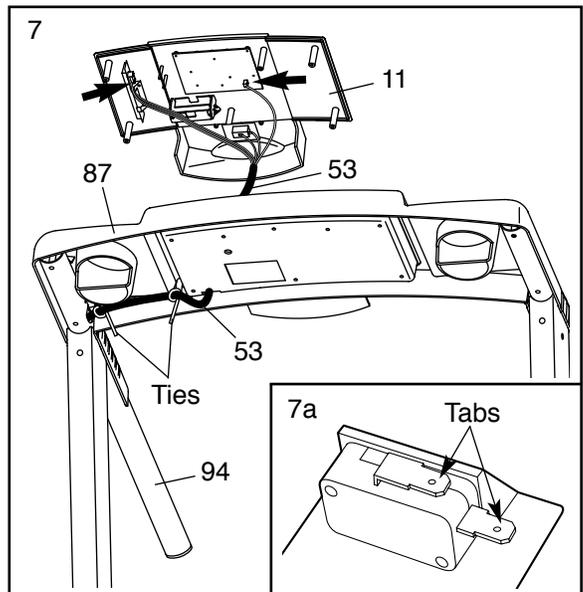
8. Set the Console (11) in the Console Base (87). Cover the Wire Harness (53) with the Wire Cover (10), and route the Wire Harness out of the hole in the side of the Wire Cover. Attach the Wire Cover to the back of the Console Base with two 3/4" Screws (5). **Make sure that no wires are pinched before you attach the Console to the Console Base.**
