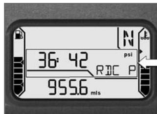
The tire inflation pressures are displayed with the lettering RDC P. The left-hand value indicates the inflation pressure of
