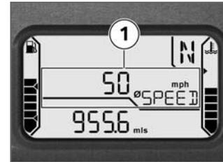
The average speed **1** is calculated based on the elapsed time since the last reset. Times during which the engine was stopped are excluded from the calculation.
