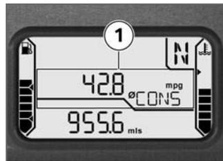
The average consumption **1** is calculated by dividing the distance covered since the last re-
