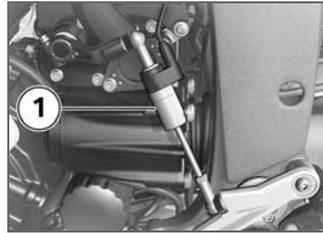
The sensor **1** in the shift linkage detects the shift request and initiates shifting support.
