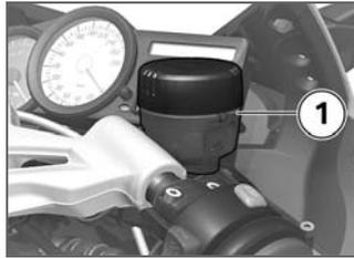
**⚠** A low fluid level in the brake reservoir can allow air to penetrate the brake system. This significantly reduces braking efficiency. Check brake fluid level regularly.◀
