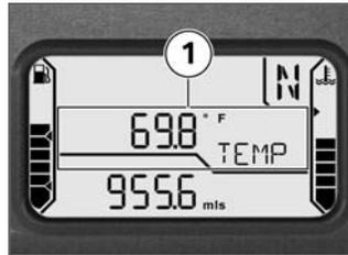
When the motorcycle is stopped, the engine heat can falsify the measurement of the ambient temperature **1**. If the influence of the engine heat becomes too great, -- is temporarily shown in the display.
