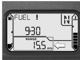
The operating range indicates what distance can still be driven with the remaining fuel. It is only displayed after the fuel reserve is reached. This distance is calculated on the basis of fuel level and average consumption. When refueling after running on reserve, make sure that you top up the tank to a level above reserve, as otherwise the sensor will not be able to register the new level. Otherwise neither the
