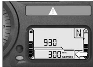
If the motorcycle is driven long distances annually, it is possible that earlier service is required. If the odometer reading for the earlier service lies within 600 miles (1,000 km), the remaining miles (kilometers) are counted down in 60-mile (100-km) steps and briefly displayed following the pre-ride check.
