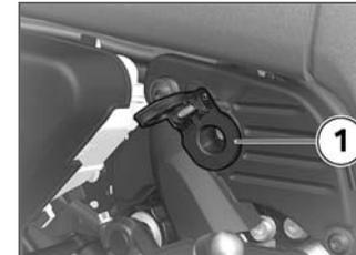
The supply to the socket **1** is cut off automatically if battery voltage is too low or the load exceeds the maximum rating.
