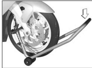
**⚠** If the motorcycle is resting on the center stand: The motorcycle is raised too far at the front, the center stand lifts off the ground and the motorcycle can tip over to the side. When raising the motorcycle, make sure that the center stand remains on the ground.◀
