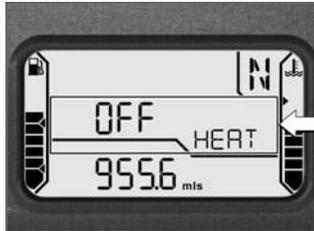
The handlebar grips can be heated at two different levels. The second level is used for fast heat-up of the grips; then the switch should be switched back
