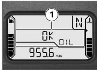
The oil level indicator **1** provides information on the oil level in the engine. It can only be displayed when the motorcycle is stopped.
