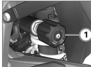
**⚠** Your motorcycle's handling will suffer if you do not match the spring-preload and damping-characteristic settings. Adjust the damping characteristic to suit the spring preload.◀
