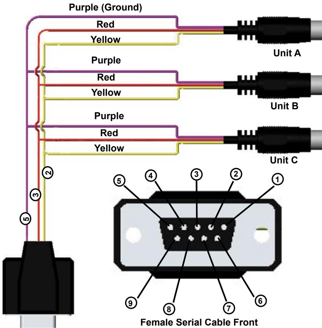
Figure 3. Typical Multiple Device (Addressable) Wiring Configuration
