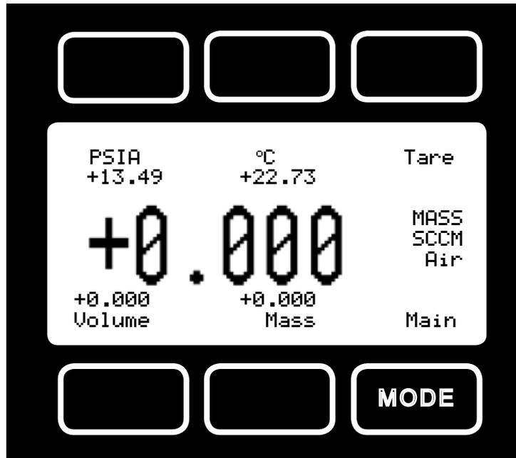
Figure 6. Main Mode Display, M Series Flow Meter
