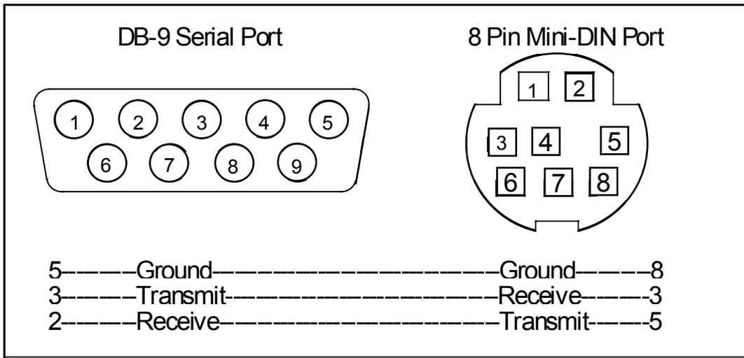
Figure 2. Mini-DIN to DB-9 Connection for RS-232 Signals
