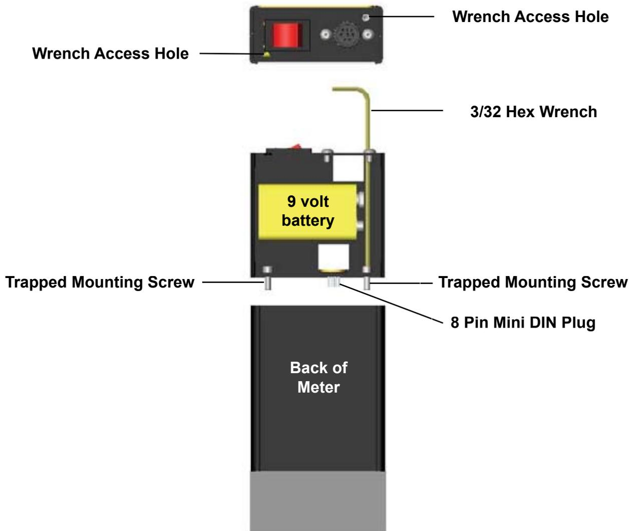
Battery Pack Installation/Removal
