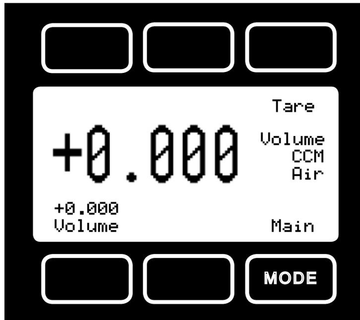
Figure 11. Main Mode Display, V Series Flow Meter
