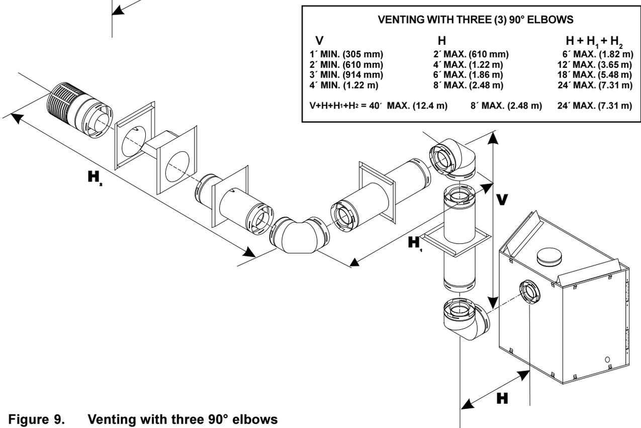
**Figure 9. Venting with three 90° elbows**
