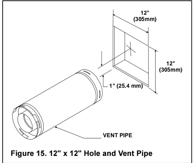
Figure 15. 12" x 12" Hole and Vent Pipe
