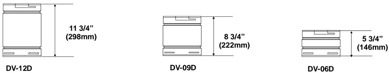
NOTE: PIPES OVERLAP  $1 \frac{3}{8}$  INCHES (34.93mm) AT EACH JOINT.
