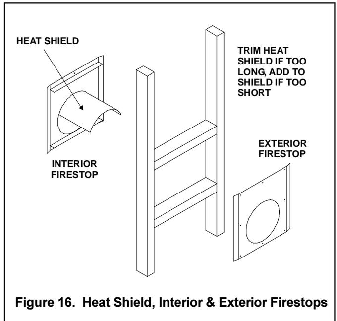
Figure 16. Heat Shield, Interior & Exterior Firestops
