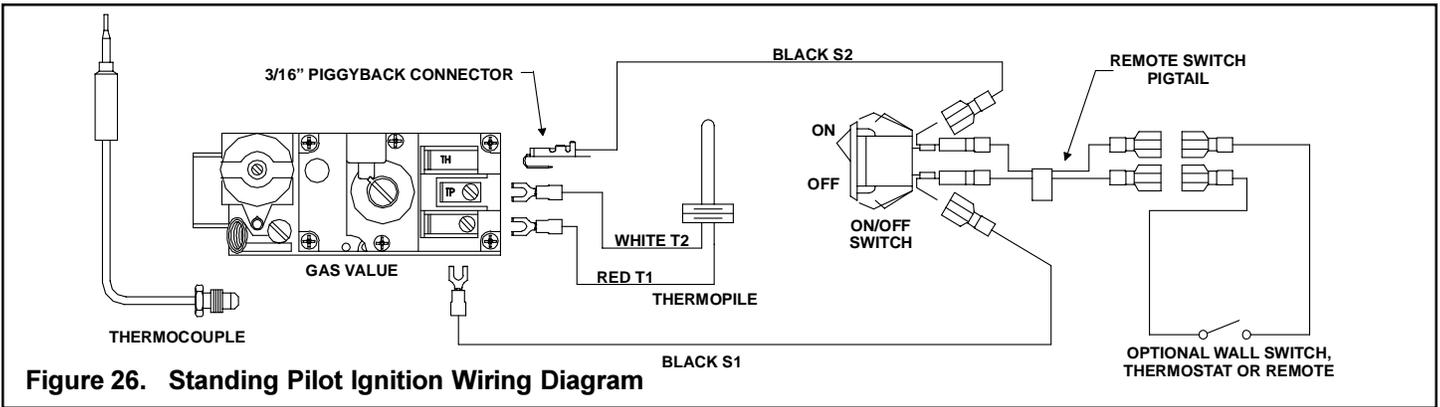
Figure 26. Standing Pilot Ignition Wiring Diagram
