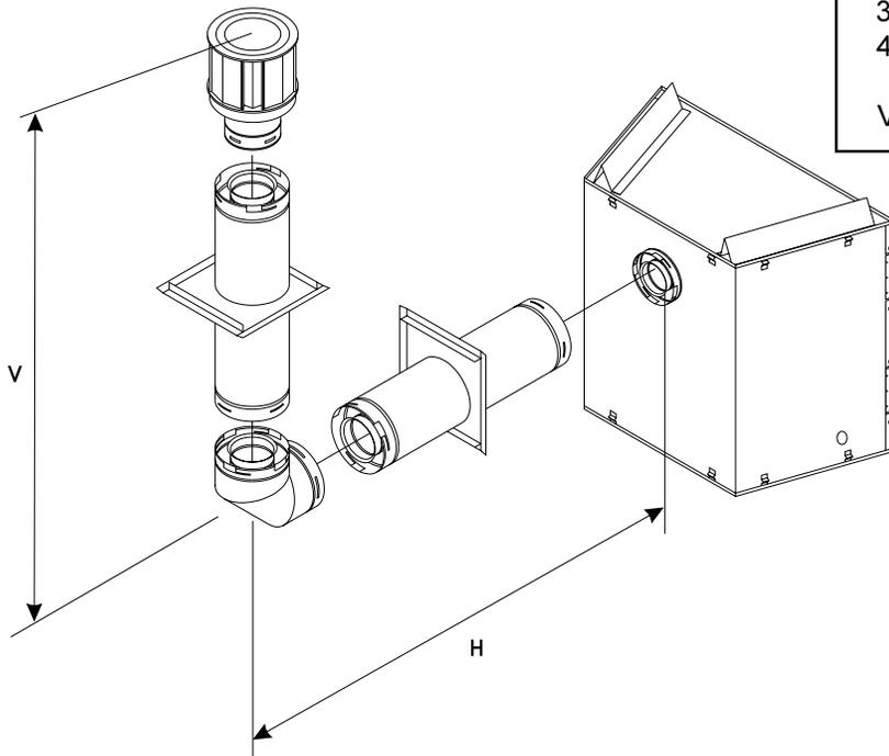
**NOTE:** On vertical venting configurations where the vertical component is over 10 feet, you may want to install the vertical baffle included in the manual bag assembly to improve flame appearance.
