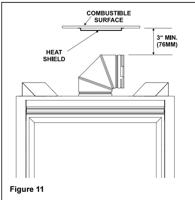
2. Fasten the shield in place using the four pilot holes provided in the part. The shield should be oriented such that the 13 1/8 inch dimension (longest dimension) is running in the same direction the elbow is pointing. The shield should be centered directly above the elbow, and positioned so that it creates a 1/2 inch airspace between the shield and the combustible surface. See Figure 12.
