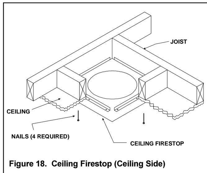
If the area above the ceiling **IS** an attic, position and secure the firestop on top of the previously framed hole.
