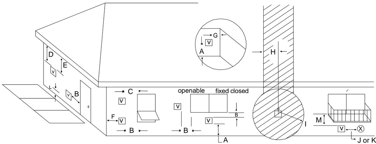
**V** = VENT TERMINAL      **X** = AIR SUPPLY INLET      [Hatched] = AREA WHERE TERMINAL IS NOT PERMITTED
