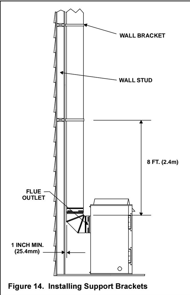
Figure 14. Installing Support Brackets
