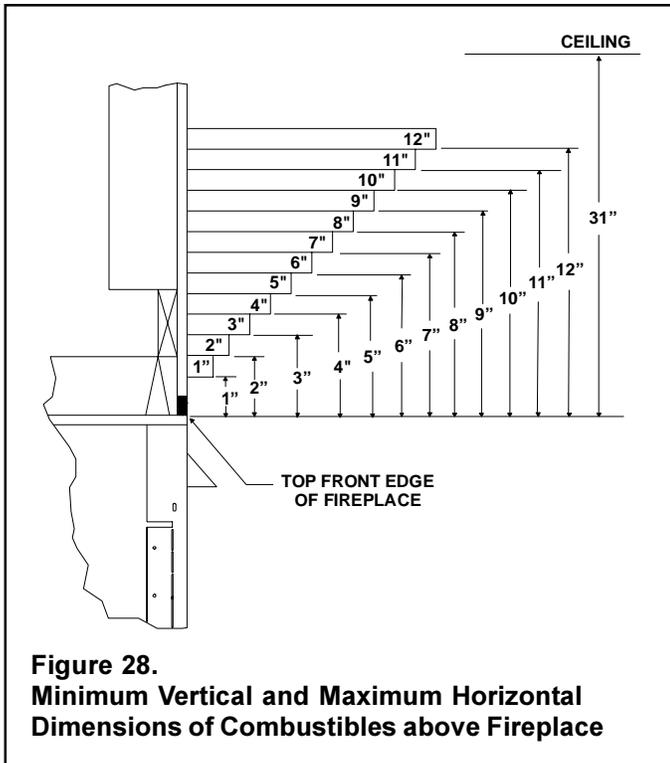
**CAUTION: IF JOINTS BETWEEN THE FINISHED WALLS AND THE FIREPLACE SURROUND (TOP AND SIDES) ARE SEALED, A 300° F. MINIMUM SEALANT MATERIAL MUST BE USED. THESE JOINTS ARE NOT REQUIRED TO BE SEALED. ONLY NON-COMBUSTIBLE MATERIAL (USING 300° F. MINIMUM ADHESIVE, IF NEEDED) CAN BE APPLIED AS FACING TO THE FIREPLACE SURROUND. SEE THE DIAGRAM BELOW.**
