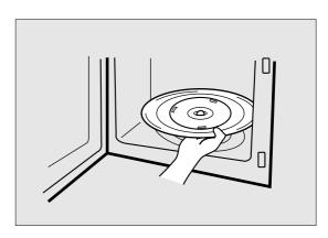
7 The roller guide and oven cavity floor should be cleaned regularly to avoid excessive noise. Simply wipe the bottom surface of the oven with mild detergent water or window cleaner and dry. The roller guide may be washed in mild sudsy water.
