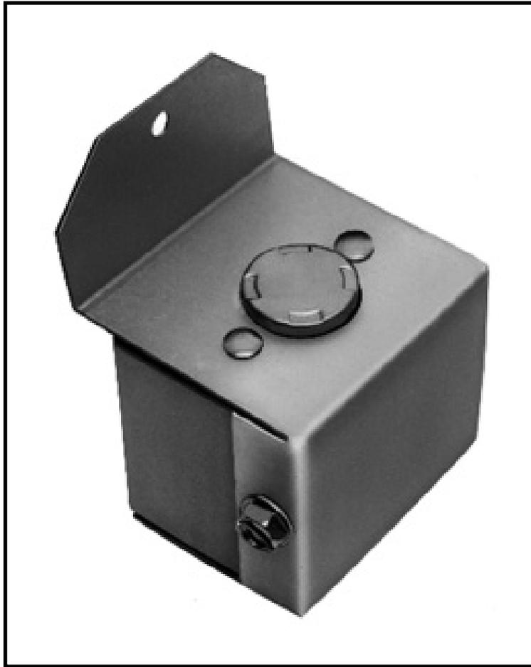
Installation of a spillage SAFETY Switch is recommended for LP and Natural gas fired systems with draft hoods, draft diverter, or gas barometric draft controls. This device is installed to detect flue gas spillage caused by a blocked flue system and/or inadequate draft. This device MUST be installed by a qualified installer in accordance with the manufacturer's installation instructions. Wiring MUST be in accordance with the National Electrical Code and applicable local codes.
