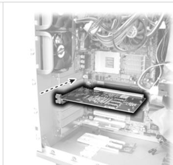
Seat the board securely into the slot.
