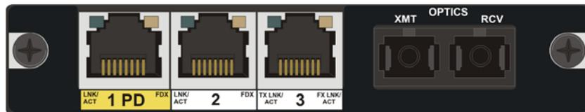
Port 2 is dedicated for high priority applications. All other RJ-45 ports provide fixed DiffServ/ToS-PRI prioritization, giving higher priority to all traffic with a VLAN TAG with PRI>4. All RJ-45 ports incorporate the Auto Cross and Auto Negotiation features. The Fiber-Optic configuration also includes the Far End Fault feature that provides notification of far-end link loss on the fiber port.
