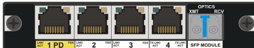
Configuration 3: One additional RJ-45 data port and one Fiber-Optic data port (SFP).
