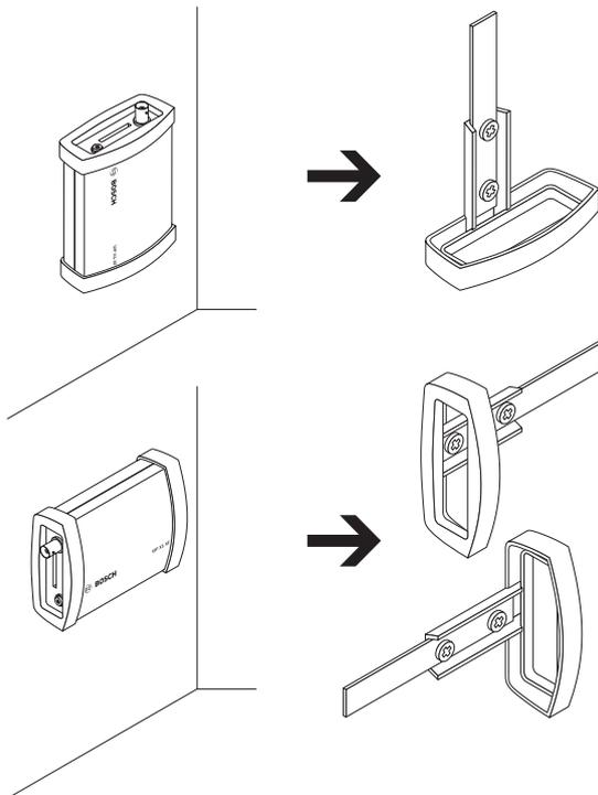
You can secure the VIP X1 XF E to any load-bearing wall using the wall-mounting panel, in either a vertical or a horizontal position.
