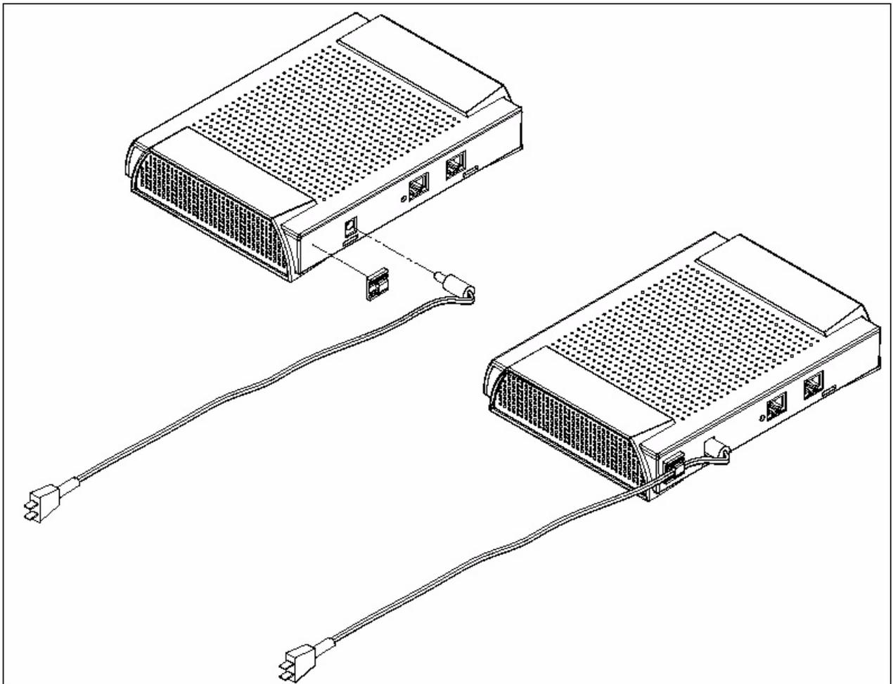
**Figure 1** Power Kit Installation
