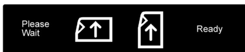
The **scanner document feed panel**, located below the scanner control panel, displays the document feed direction.
