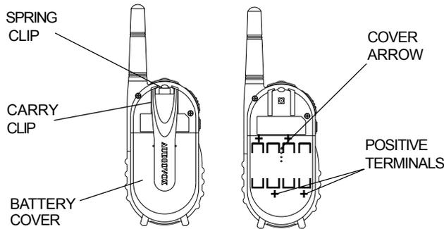
1. Using thumb, press down on battery cover at arrow and slide cover down to open.
