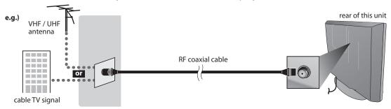
\* Once connections are completed, turn on the unit and begin initial setup. Channel scanning is necessary for the unit to memorize all available channels in your area. Refer to "Initial Setup" on page 17.
