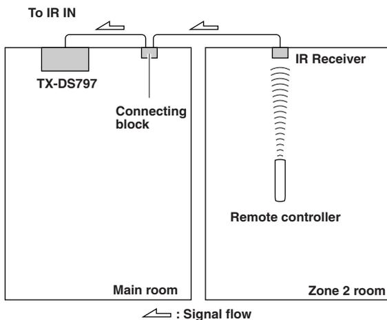
Make connection as shown below. Do not plug the equipment into the power source until the connection is complete.
