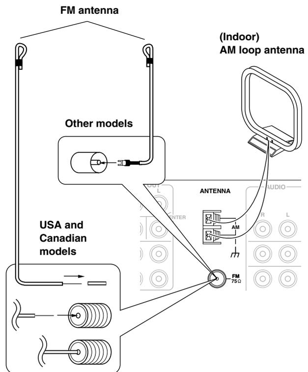
Strip away the insulation from the end of the cable, then fully insert the stripped end of the cable.
