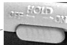
**NOTE:** The Hold Switch must be **OFF** to power on the RioVolt.
