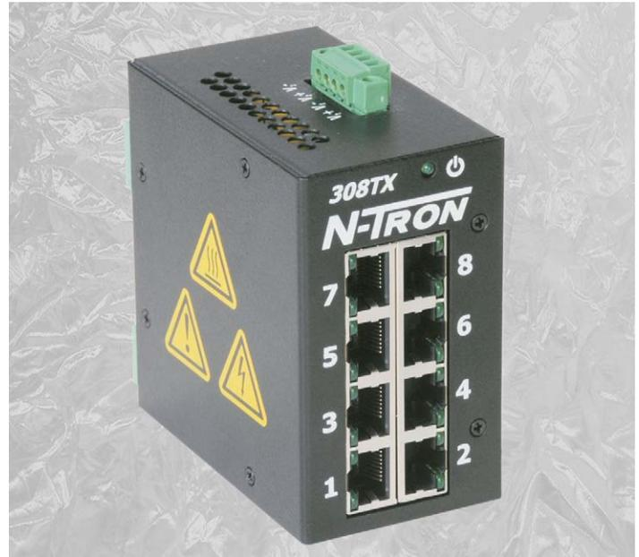
to a climate controlled environment. The 308TX has extended operating environmental specifications to meet the harsh needs of the industrial environment. For cost savings and convenience the 308TX can be DIN-Rail mounted alongside Ethernet I/O or other industrial equipment.
