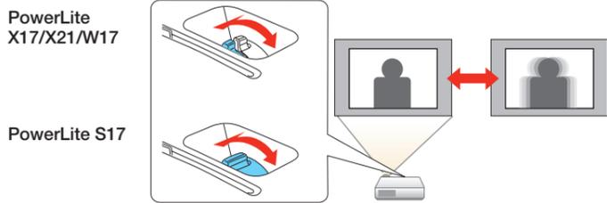
5 If your image looks like or , you may have placed the projector off to one side of the screen at an angle. Place the projector directly in front of the center of the screen, facing the screen squarely. If you can't move the projector, use the horizontal keystone slider to correct the image.
