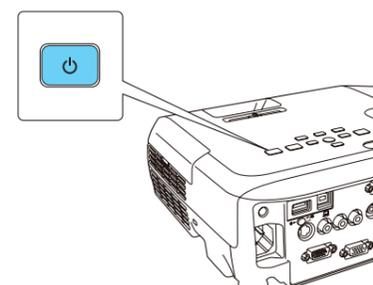
**Note:** To shut down the projector, press the power button twice, then unplug it. You don't have to wait for the projector to cool down.
