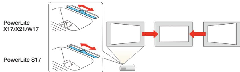
6 Your projector automatically adjusts images that look like or , but if necessary you can press the or button on the projector to correct it.
