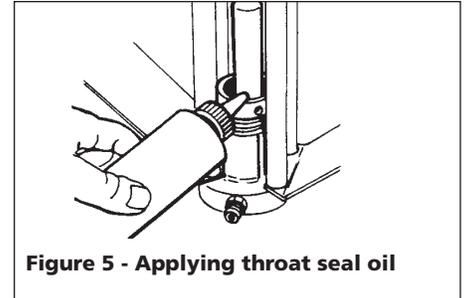
**Figure 5 - Applying throat seal oil**
