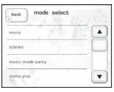
Touching the **up** or **down arrows** scrolls through the list of modes. Touch any mode (that isn't grayed out) to select it. The SSP-800 processing changes to the newly-selected mode. Press the **Back** button to return to the Home page. The available modes are described in Table 2.
