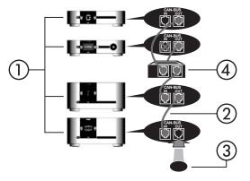
NOTE: Daisy chain must be terminated with CAN-Bus Terminator.
