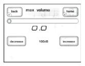
NOTE: The volume knob itself does not set the maximum volume; you must set the maximum volume level in this Max Volume setup menu.
