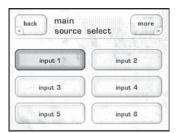
Touch any **input** button on the touchscreen to select it as the current input. If the input you want to activate is not on this screen, press the **More** button for the next page of input options. Or, press the **Back** button to return to the previous page.
