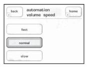
This volume control is specifically for use with automation control systems. Such control systems can vary in how quickly they repeat ramped volume commands. By first selecting a suitable volume control speed on the SSP-800 Surround Sound Processor, the programming required to tailor the speed from the control interface is simplified.
