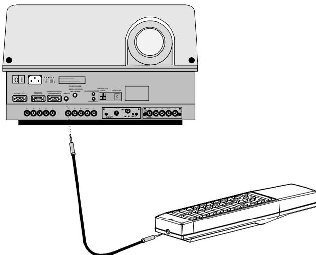
Plug one end of the remote cable in the connector on the bottom of the RCU and the second side in the connector in the front panel of the projector labelled 'REMOTE'.
