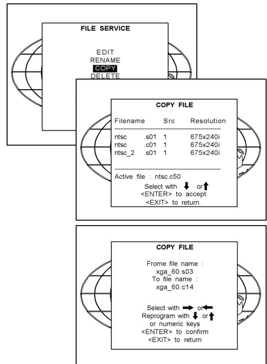
The first character is highlighted. Push the control disc to the right or to the left to select the desired character. Change that character by pushing the control disc up or down. Numeric characters can be entered directly with numeric keys on the RCU. Press **ENTER** to confirm. The copied file is entered in the list of files. Press **EXIT** to return to the Copy selection menu. No copies are made.
