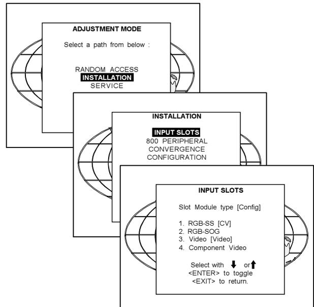
When using an RCVDS 05 with a 5 cable output module, connect these 5 cables to this fixed 5-input slot (slot2) of the projector. All sources of the RCVDS can now be accepted by the projector.
