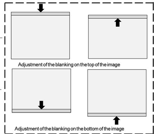
Correct by pushing the control disc up or down
