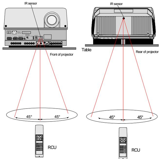
When using the wireless remote control, make sure you are within the effective operating distance (30m, 100ft in a straight line). The remote control unit will not function properly if strong light strikes the sensor window or if there are obstacles between the remote control unit and the projector IR sensor.
