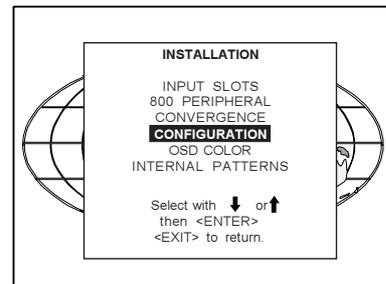
The actual selected configuration will be highlighted. Push the control disc forward or backward to select the corresponding configuration with regard to the projector environment. Press **ENTER** to confirm your selection.
