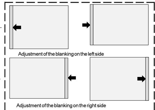
Correct by pushing the control disc to the right or to the left
