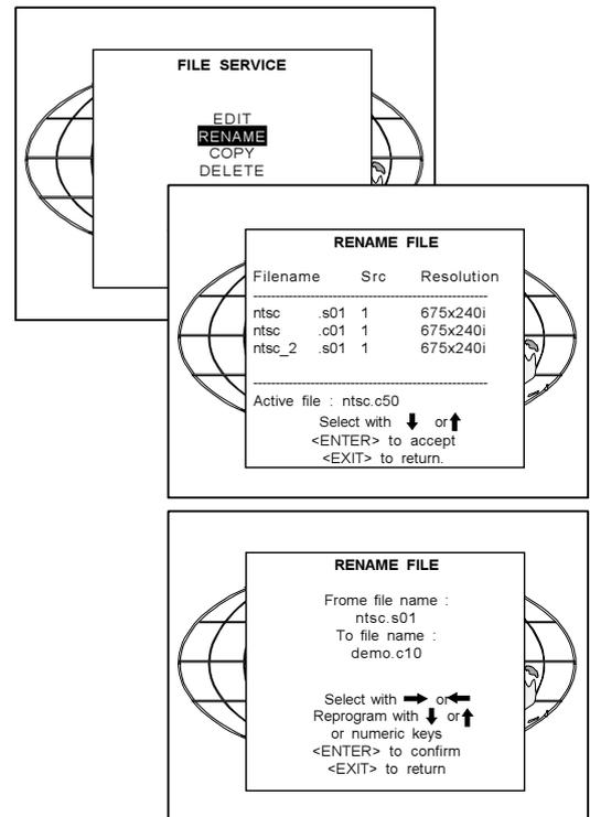
The first character is highlighted. Push the control disc to the right or to the left to select the desired character. Change that character by pushing the control disc up or down. Numeric characters can be entered directly with numeric keys on the RCU. Press **ENTER** to confirm. The renamed file is entered in the list of files. Press **EXIT** to return to the Rename menu selection. No changes are made.
