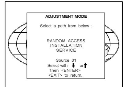
Some items in the Adjustment mode are password protected. While selecting such an item, the projector asks to enter your password (Password protection is only available when the password strap on the controller module is ON, see 'Change password' in chapter 10 : 'Service mode').
