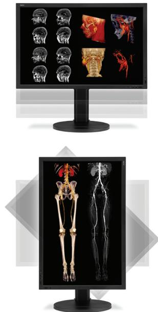
The MD304MC's design allows you to adjust the display to your exact ergonomic preferences. In addition to tilt and swivel functionality, the height adjusts up to 190mm, and the display pivots between landscape to portrait orientations.
