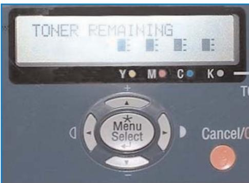
Use the Display key on the all-in-one control panel to display the toner "gas gauges."
