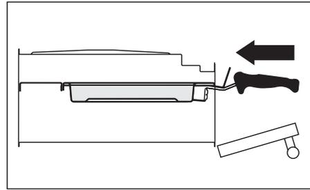
For best results preheat for 2 minutes with the broiler pan in position. After placing your food on the broiler pan grid, slide the broiler pan onto the side supports. Adjust the heat to suit by turning the knob.
