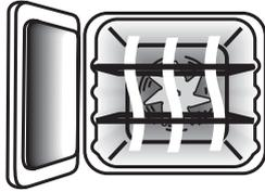
The left hand oven is a Multi-function oven. As well as the oven fan and fan element, it is fitted with two extra heating elements, one visible in the top of the oven and the second under the oven base. Take care to avoid touching the top element and element deflector when placing or removing items from the oven. For more detail on this oven see the section 'Multi-function oven'.
