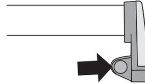
Remove the 2 cross headed screws that were hidden by the hand rail end brackets.
