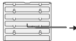
Lift up the front of the rack so the back of the rack will pass under the rack stop and then pull the rack forward.
