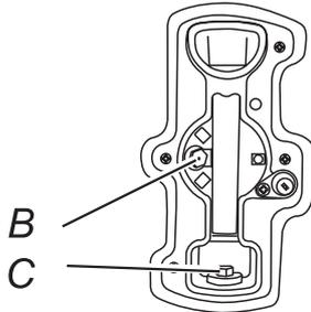
A orifice, B internal injector, C external injector
