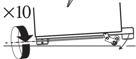
Make sure you lower **BOTH REAR ROLLERS**. There are two adjusting nuts, one for each roller, at both the front bottom corners of the range.
