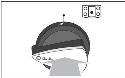
If, when you let go of the control knob, the burner goes out, the safety device has not held in. Turn the control to the off position and wait one minute, then try again this time holding in the control knob for slightly longer.
