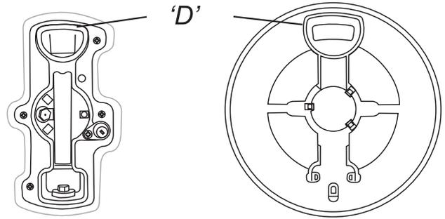
Turn the head until the 'D' matches the one on the burner base. Turn the head over and place it on the burner base. To fit the small inner burner, find the larger electrode notch in the burner rim. Line this up with the white ignition electrode and place the inner burner on the large base ring.
