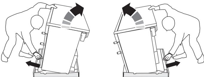
Repeat from the front and remove the front half of the polystyrene base.
