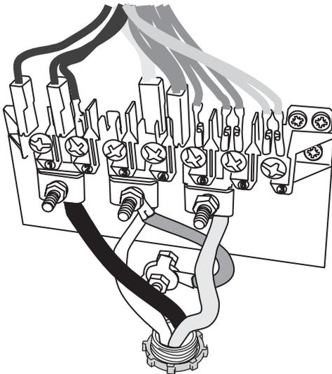
The neutral or ground wire of the power cord must be connected to the neutral terminal located in the center of the connector block. The power leads must be connected to the outside terminals.
