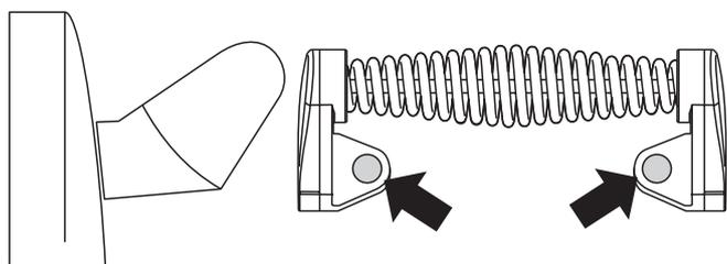
Fit the plastic blanking plugs to the fixing holes.
