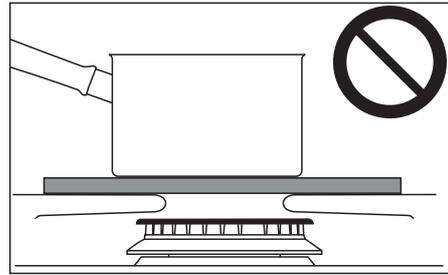
Simmering aids, such as asbestos or mesh mats, are **NOT** recommended. They will reduce burner performance and could damage the grates.
