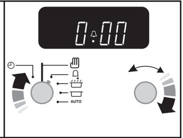
You can turn the knob back to the (⌚) manual setting to keep an eye on the time of day or leave it in the (🕒) minute minder position as the time ticks down.
