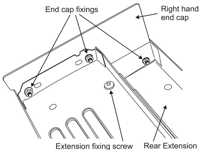
They are held in place by three fixing nuts on the inside face.
