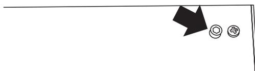
Remove the 4mm Hex headed screws from the top corners of the fascia.
