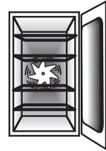
The fan in the right hand Tall oven circulates hot air continuously, which means faster more even cooking. The recommended cooking temperatures for a fanned oven are generally lower than a non-fanned oven.
