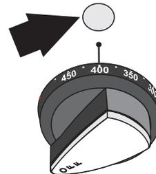
The oven heating light will glow until the oven has reached the temperature you selected. It will then cycle on and off during cooking.
