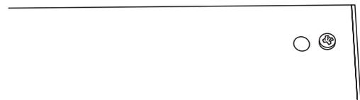
Open the oven door & or broiler door and remove the fixing screws underneath the control panel.
