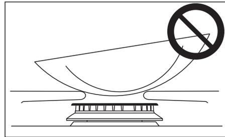
Avoid using unstable and misshapen pans that may tilt easily and pans with a very small base diameter e.g. milk pans, single egg poachers. The minimum pan diameter recommended is  $4\frac{3}{4}$ ".
