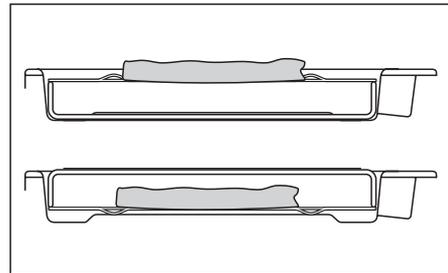
The broiler pan grid can be turned over to give two cooking positions.
