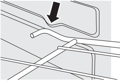
To refit the rack, line up the rack with a groove in the oven side and push the rack back until the ends hit the rack stop. Lift up the front so the rack ends clear the rack stops, and then lower the front so that the rack is level and push it fully back.
