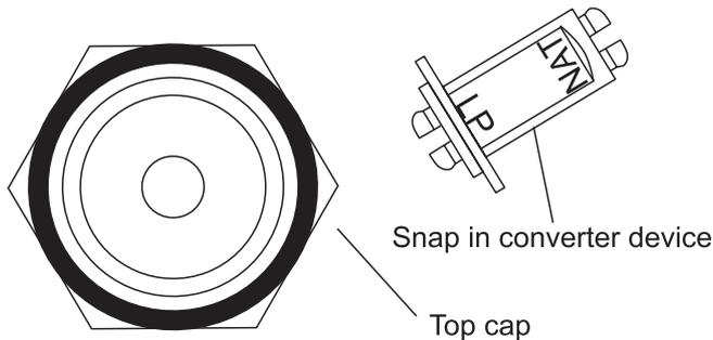
In the base of the brass top is a plastic snap in converter device.
