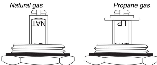
To convert the regulator snap the device out of the top and refit the other way up. The snap in converter device is marked to show which gas it is set for. Make sure the device is secure in the top cap and refit the cap to the regulator.
