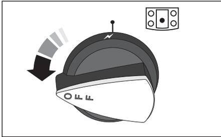
Keep holding the knob pressed in to let the gas through for few seconds. The igniter should spark and light the gas.
