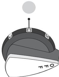
Turn the function selector control to a cooking function. This is the fan oven setting.
