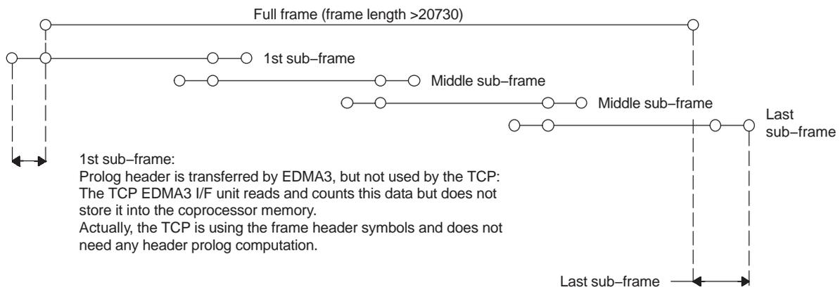
A full sub-frame including the header and tail prolog is transferred by EDMA3 but the totality is not used by the TCP.
