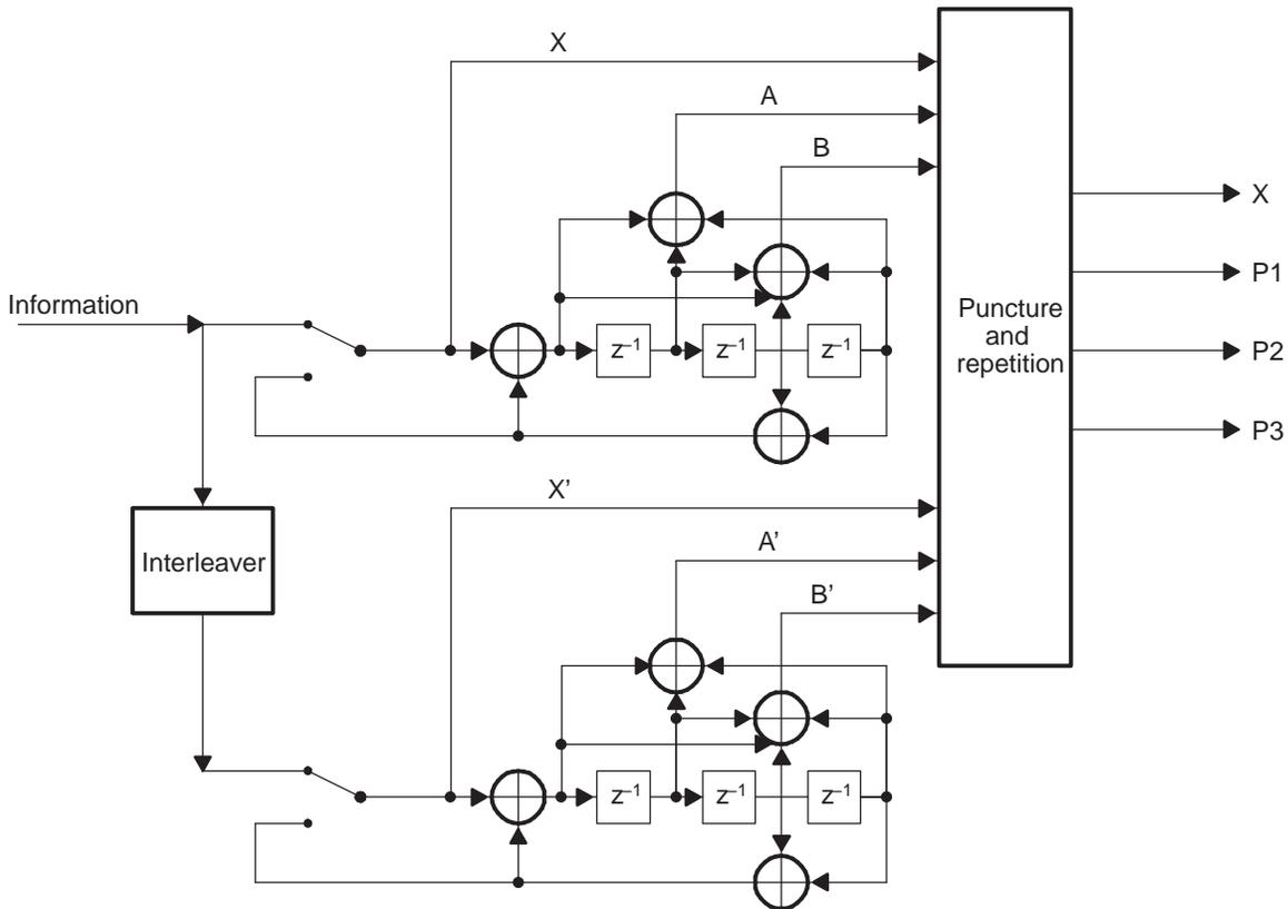
Switches in upper position for information bits and in lower position for tail bits
