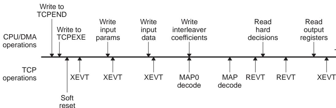
**Figure 101. TCP2 Events Generation in Shared-Processing (SP) Mode**
