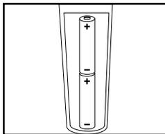
Insert two LR 06 1.5 V batteries.
