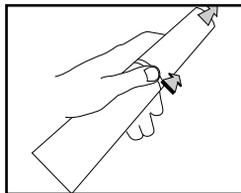
To open the cover, press as indicated and push in the direction of the arrows.
