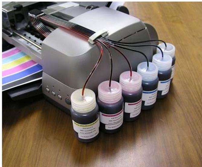
Insert the tubing into the tube clip and close it until it snaps shut. Don't pinch any of the tubes.
