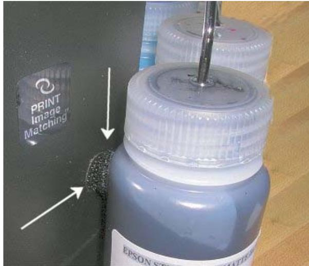
*Velcro attaches bottles to printer
