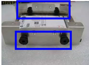
Step 4: Put the rubbers into indentations to fix the whole HDD brackets with HDD on HDD box
