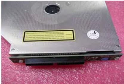
Step 3: Fasten the CD-ROM module on the on the chassis and plug the cable
