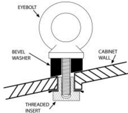
For side inserts, use 6 mm x 1mm pitch x 25.4 mm thread length steel forged shoulder eyebolt.
