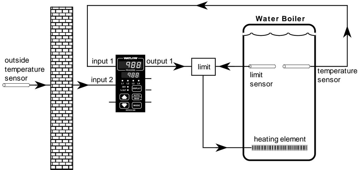
Figure 9.7 - Water boiler with differential control.
