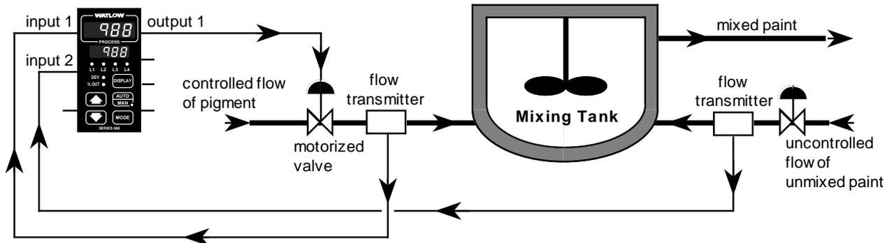
**Figure 9.13 - Mixing tank with ratio control.**
