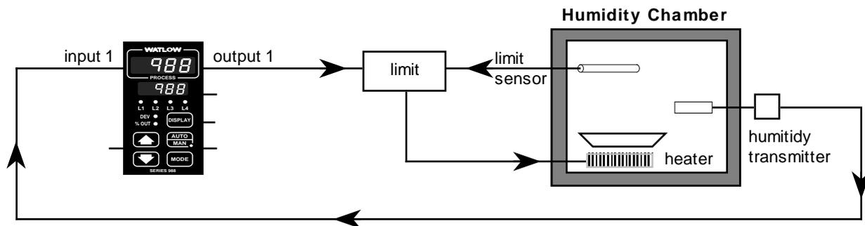
Figure 8.13b - Humidity chamber with input filtering.
