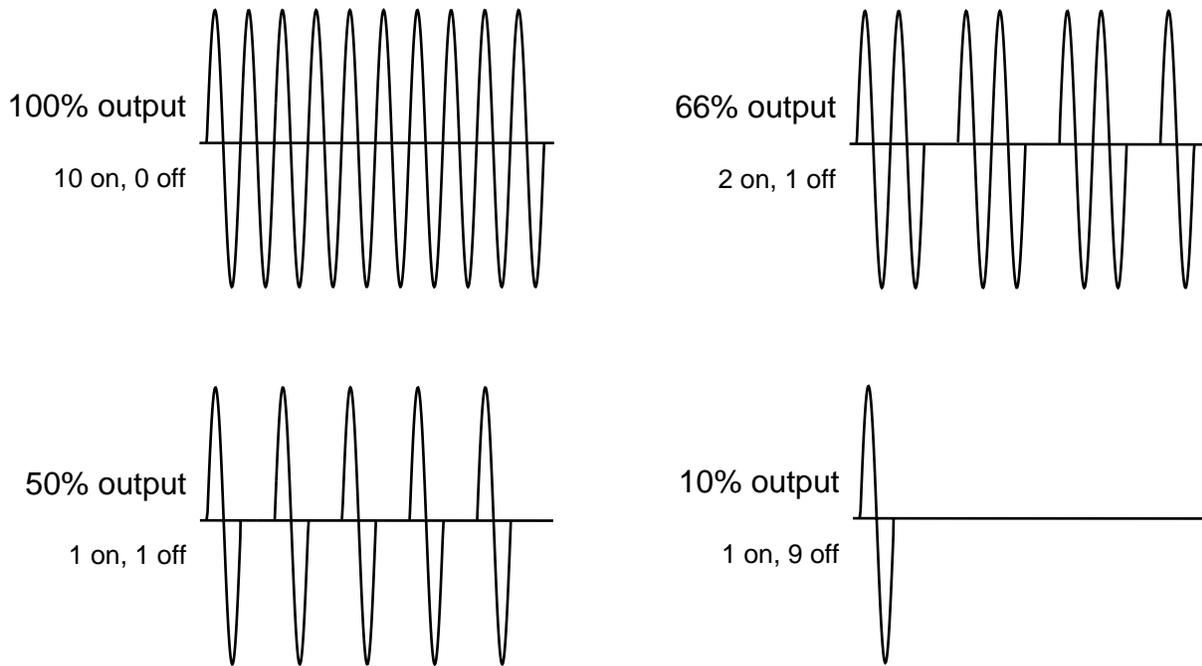
Figure 8.3a - Sine waves of burst fire settings.
