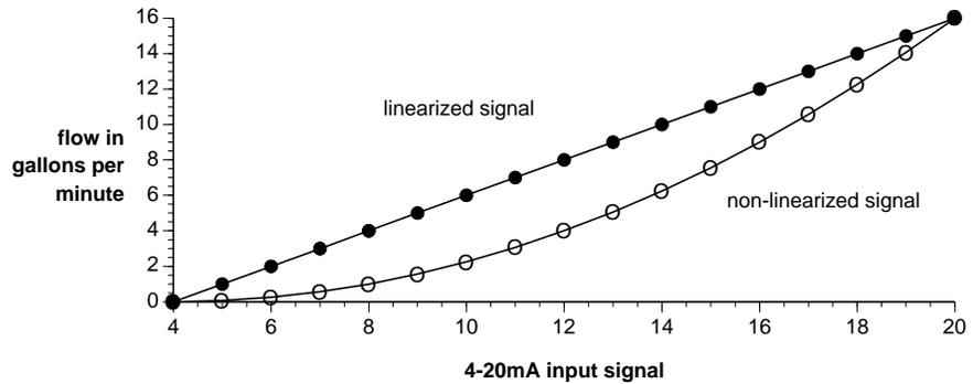
Figure 8.15a - Graph of linearized signal.
