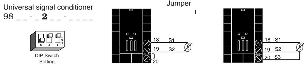
**Figure 2.9c — 0-5V<sub>DC</sub>, 1-5V<sub>DC</sub> or 0-10V<sub>DC</sub> Process**
