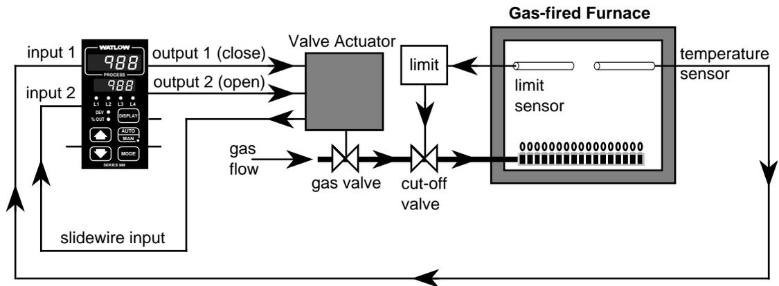
Figure 8.23 - Gas-fired furnace with slidewire feedback.
