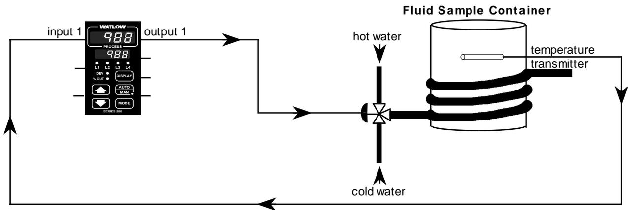
Figure 9.11 - Fluid sample container with duplex control.
