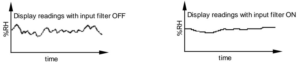
Figure 8.13a - Display readings with input filtering.
