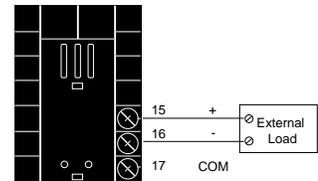
**Figure 2.13c — 0-20mA and 4-20mA Process**
