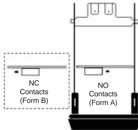
**Figure 7.5 - Alarm jumper location.**
