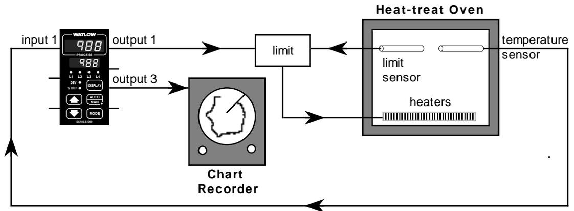
Figure 8.21 - Heat-treat oven with retransmit.
