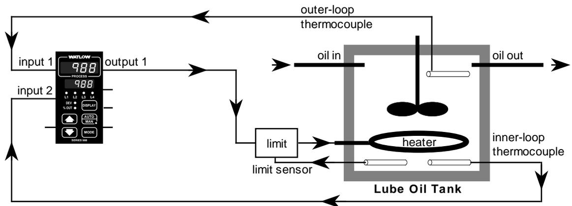
**Figure 9.5 - Lube oil tank with cascade control.**
