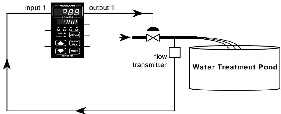
Figure 8.15b - Waste-water treatment with input linearization.
