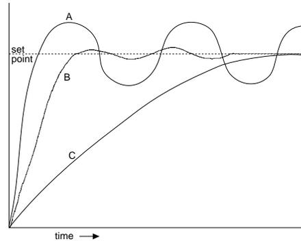
Figure 9.2a - System heat-up profiles using three different control methods.
