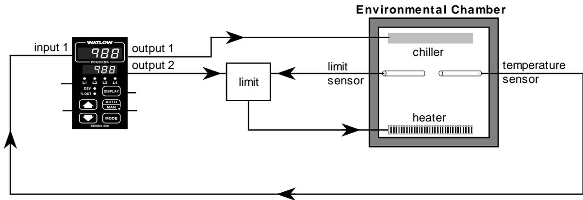
Figure 8.7b - Environmental chamber with dead band.
