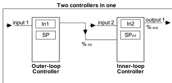
Figure 9.2b - The cascade feature allows one Series 988 controller to internalize the functions of two controllers.
