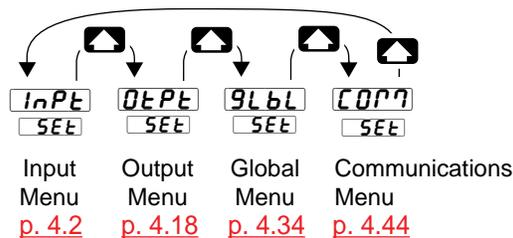
Figure 4.1 - Navigating the Setup Menus.
