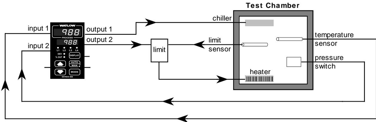
**Figure 9.9 - Test chamber controlled with dual PID sets.**
