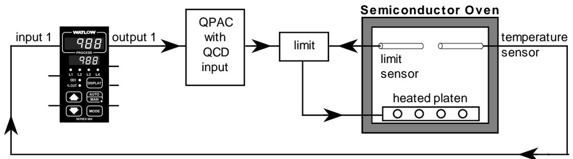
Figure 8.3b - Semiconductor oven with burst fire.
