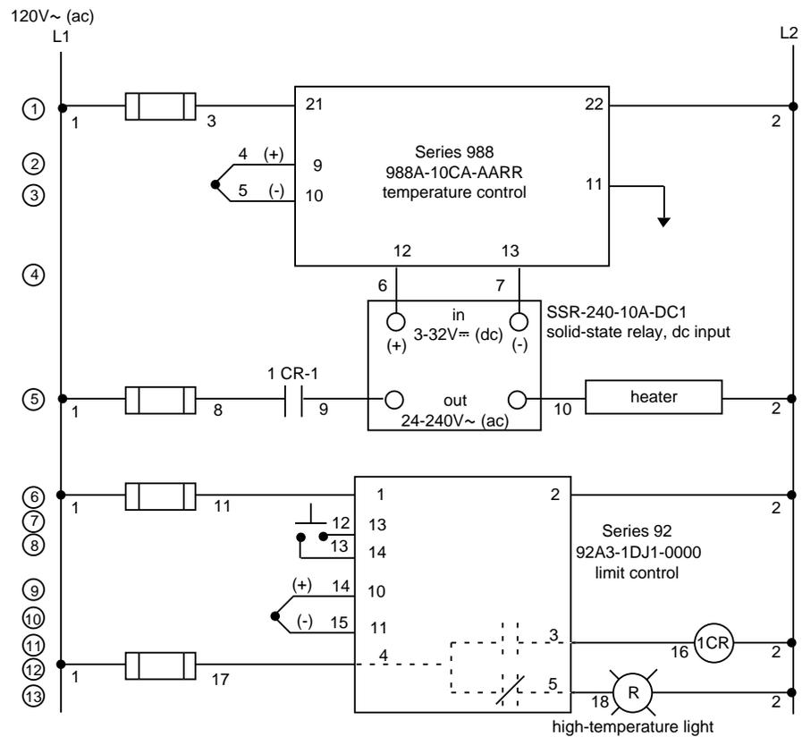
Figure 2.6 - System wiring example.
