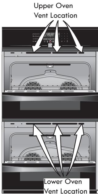
**CAUTION** Some models are equipped with a blower which runs in baking and self-cleaning mode to keep all internal components at a cool temperature. The blower may keep running even if the oven has been turned off, until the components have cooled down. On 30" double wall ovens, the blower in both ovens will start when using one of the ovens in self-clean mode.
