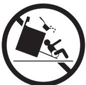
• See Installation Instructions. To reduce the risk of tipping, the wall oven must be secured by properly installed anti-tip bracket provided with the wall oven. Refer to the Installation
