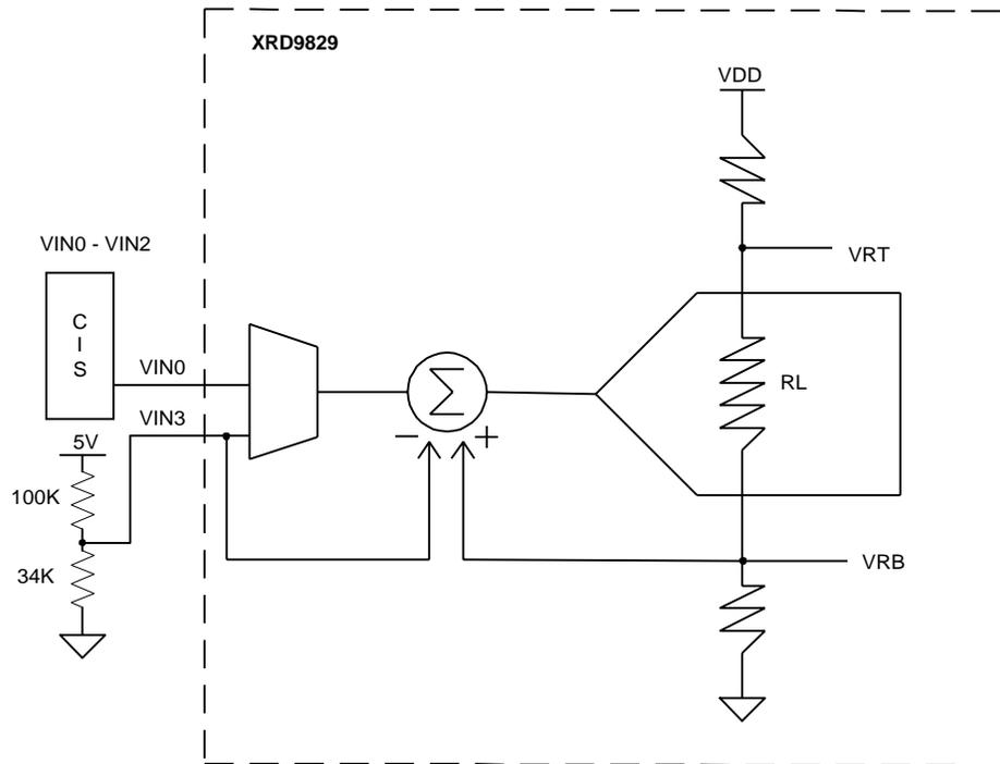
**Figure 7. Simplified Block Diagram Showing Global Offset Adjustment by XRD9829 Using External Resistor Ladder**
