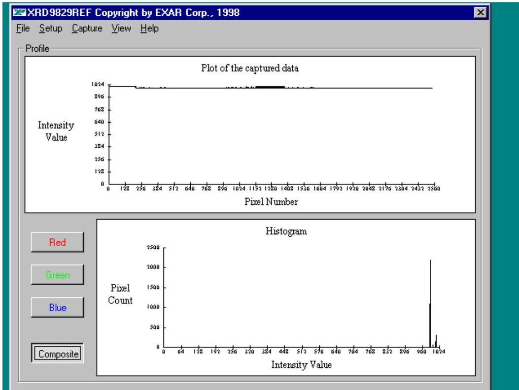
**Figure 11. White Target Scan After Gain Adjustment**
