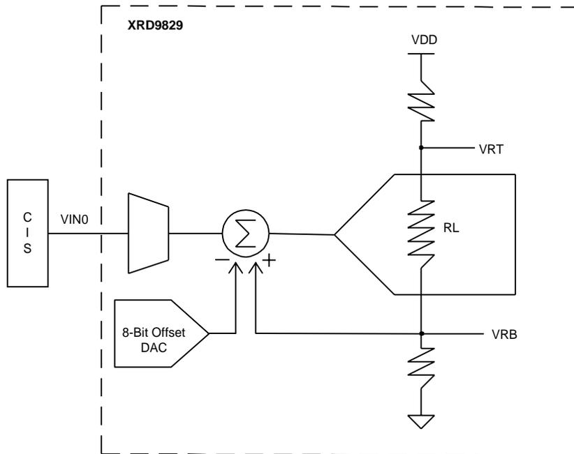
**Figure 9. Simplified Block Diagram Showing Fine Offset Adjustment by XRD9829**
