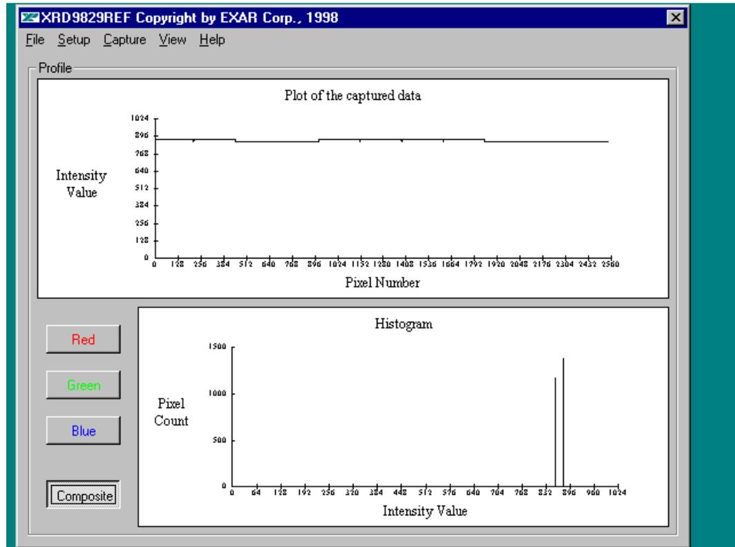
**Figure 10. White Target Scan Without Gain Adjustment**
