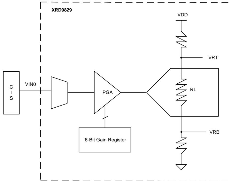
**Figure 12. Simplified Block Diagram Showing Gain Adjustment by XRD9829**
