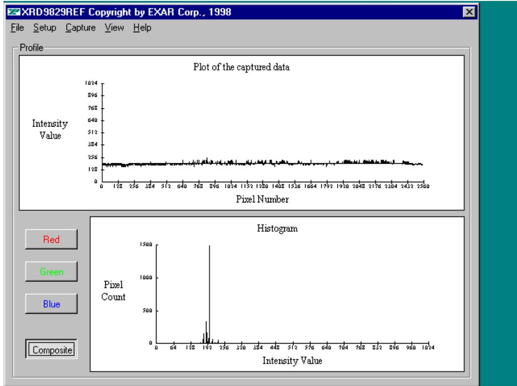
Figure 6. Black Target Scan After Global Offset Adjust
