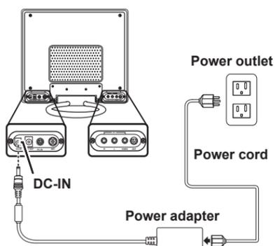
1. Connect the power cord to the power adapter as illustrated.
