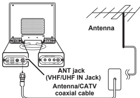
1. Connect one end of the VHF/UHF (Antenna) or CATV cable to ANT Jack (VHF/UHF IN Jack) on the back of the TV.
