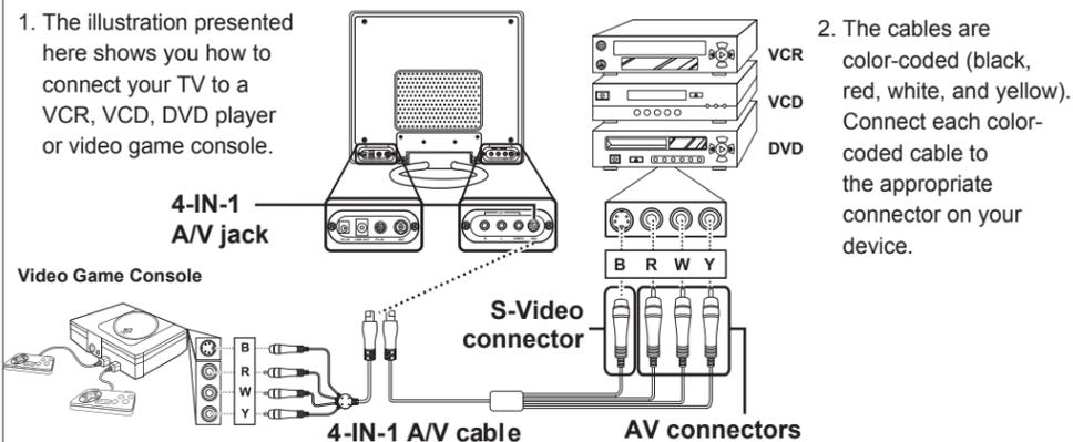
2. The cables are color-coded (black, red, white, and yellow). Connect each color-coded cable to the appropriate connector on your device.
