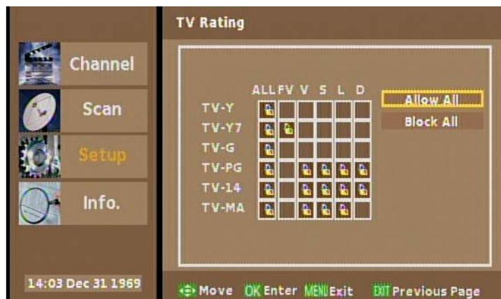
To control or change blocking for any specific setting, Press the  $\Delta/\nabla$   $\triangleleft/\triangleright$  keys to move to any box and Press OK to confirm the selection.
