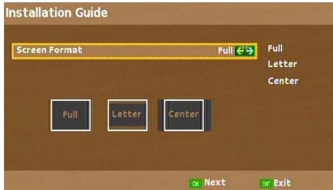
The default setting for the Screen Format is Full mode. Press Left/Right to change the Screen Format: Full, Letter, Center. Press OK to go to the next page.
