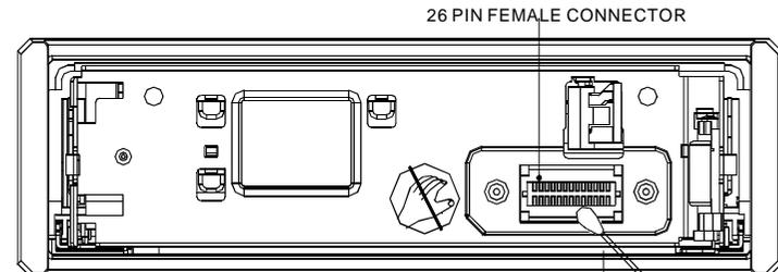
26 PIN FEMALE CONNECTOR: when there is some dirt on the connector, please wipe it away from the connector.
