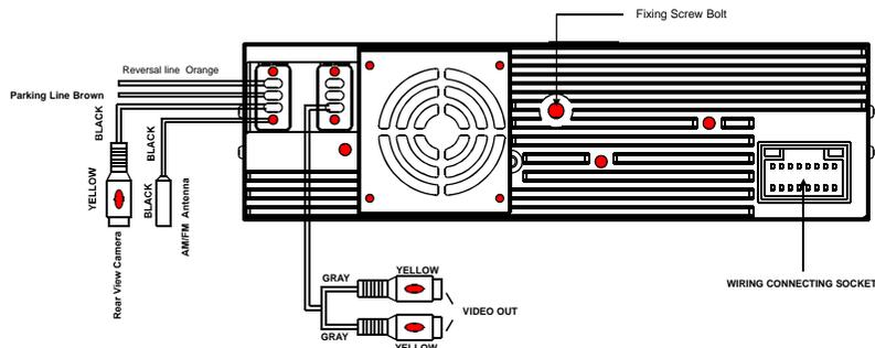
Note: 1. after connecting the Parking Line, the video on the small monitor of the front panel will display only after braking the car.
