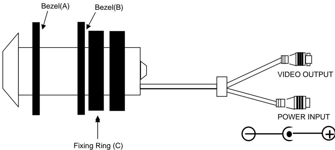
1. Place bezel(A) on the camera and then put the camera through the door.
