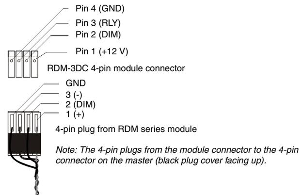
FIG. 2 Connecting the RDM-3DC and AMX Lighting Master
