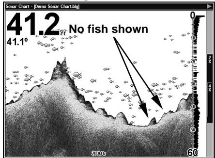
Figures 1A and 2A (left) show Sonar Page in normal chart mode. Figures 1B and 2B (right) show the same underwater scene with Fish I.D. turned on. Note how arches are replaced with symbols.
