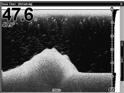
These figures show results of different sensitivity levels on the same location. Fig. 1: Sensitivity at 88 percent. Typical of full auto mode. Fig. 2: Sensitivity set at 75 percent. Fig. 3: Sensitivity set at 50 percent. Fig. 4: Sensitivity set at 100 percent.
