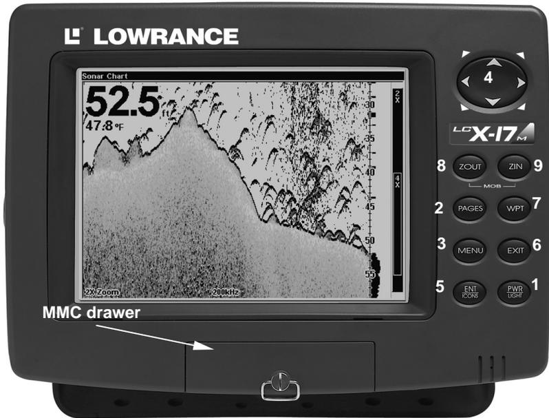
**LCX-17M sonar/GPS unit, front view, showing sonar screen, keyboard and access door for the MMC compartment.**
